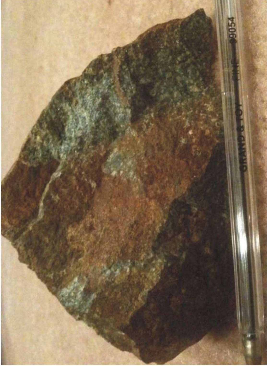
Figure 11: Plagioclase porphyritic andesite with iron oxide stained fracture surfaces and approximately 5% pyrite by volume. "Sample B" collected from immediately west of POW occurrence.
