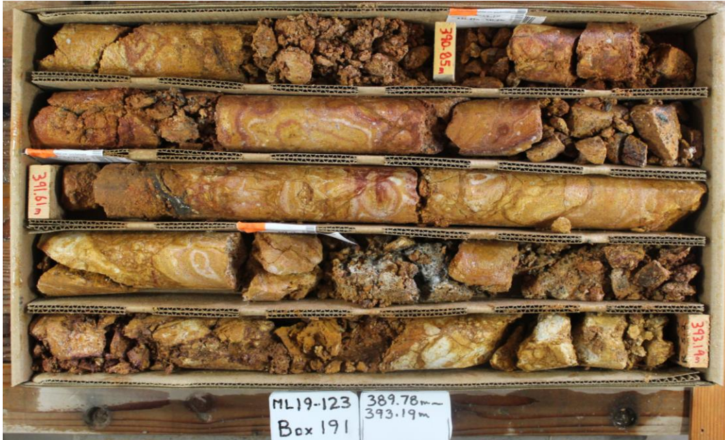
Figure 3. Drill Hole ML19-123CT Core Photo (3.41m @ 13.3 g/t Au & 2.1 g/t Ag)
